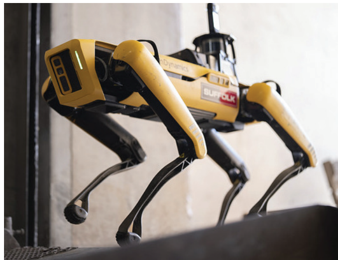
FIGURE 4 | Automatic schedule update with computer vision and robotics – SPOT walkthrough at an airport
